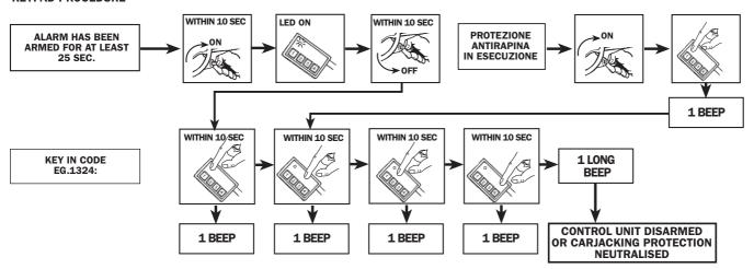
WARNING: if the wrong code is keyed in 3 times, the control unit will be blocked for 10 minutes to prevent attempts to acquire the code.
